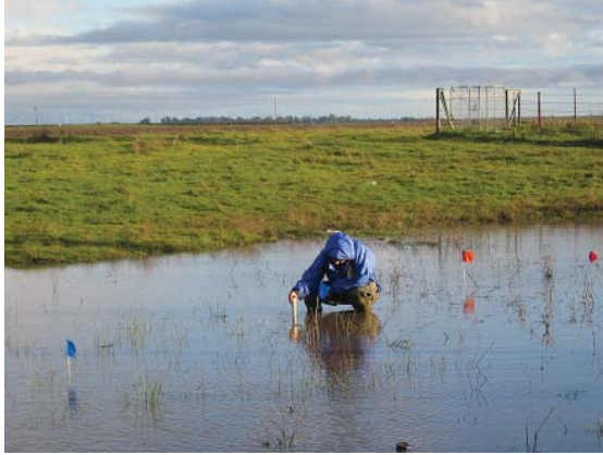
Figure 5. We used water quality meters to measure temperature, pH, conductivity, and dissolved oxygen during each site visit (photo: Pool 53, 3/3/06).
