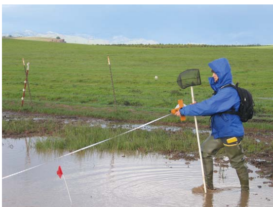
Figure 3. We measured the length of the long axis and its perpendicular axis during each site visit (photo: Pool 29, 3/3/06).
