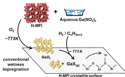
Figure 1.3.2-1. Synthesis of Ga/H-MFI via incipient wetness impregnation of H-MFI with aq. \text{Ga}(\text{NO}_3)_3 and subsequent dispersion and gas-phase ion-exchange of Ga upon exposure of impregnated zeolitic materials to \text{H}_2 or alkane reactants at temperatures > 700 K.
