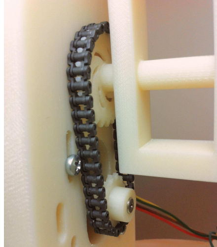
Fig. 5. Close-up view of rotating arm that is actuated by plastic chain; the chain is attached to a second smaller sprocket, which is coupled to stepper motor.
