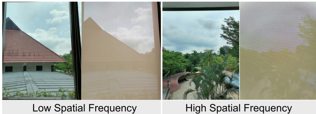
Figure 6 Comparison between two views under the same weather and time of day: both when the windows were unobstructed and when fabric roller shades were drawn. One view shows a nearby building that produce low spatial frequency content (left) and the other view has more nature (greenery) that produces high spatial frequency content (right)
