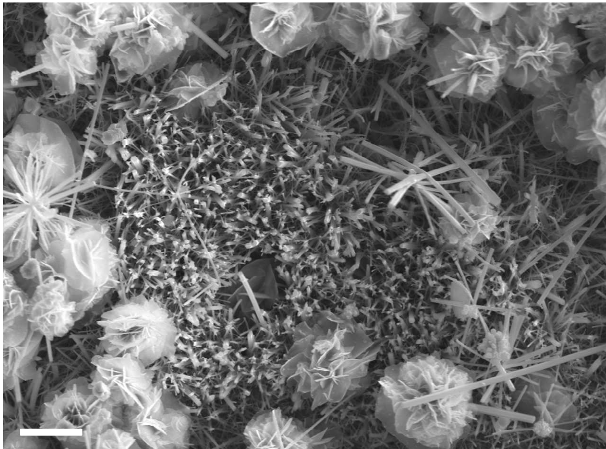
1270 1271 Figure 19: Ex-situ SE SEM images of hydrating \text{C}_4\text{A}_3 particles plus 10% solid CH in a 1272 saturated CH- \text{C}\text{H}_2 solution, liquid/solid = 50 ml/g. Hydration time was 2 hours. Accelerating 1273 voltage of 15.00 kV, a probe current of 248 pA, working distance of 13.0 mm, and scale bar is 1274 10 \mu\text{m} .
