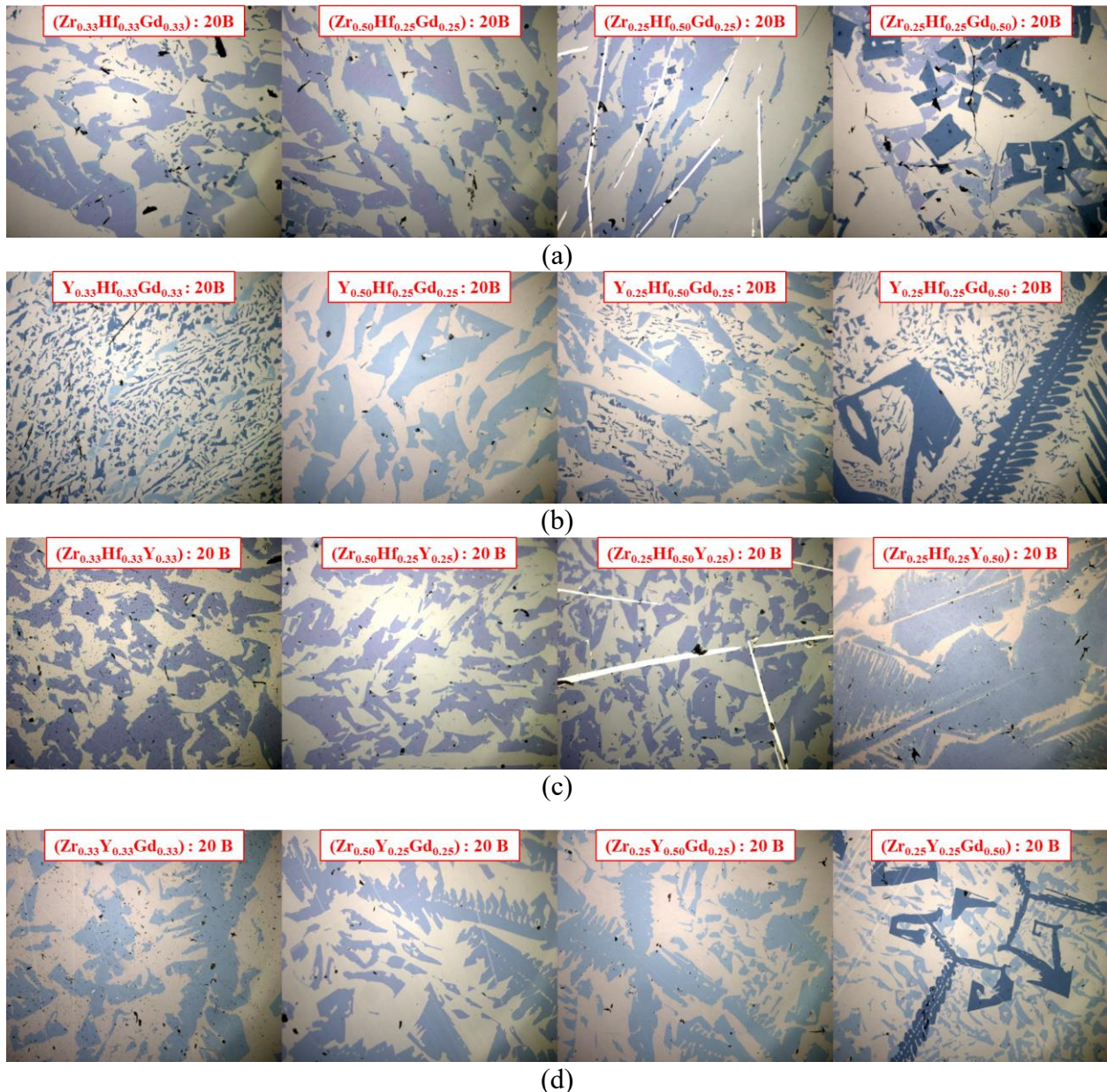
Figure 5-6. Optical images of the polished surfaces for: (a) (Zr_{1-x-z}Hf_xGd_z) : 20B ; (b) (Y_{1-x-z}Hf_xGd_z) : 20B ; (c) (Zr_{1-x-z}Hf_xY_z) : 20B ; (d) (Zr_{1-x-z}Y_xGd_z) : 20B , where x and z = 0.25, 0.33 and 0.50 . In all cases the dodecaboride MB_{12} phases exhibit a color from the blue-violet range, hexaboride MB_6 phases exhibit a deep blue color, diboride phases (white streaks) are colorless, while other areas correspond to the boron rich (also colorless) phases: MB_{50} (for Zr and Hf) and MB_{66} (for Y and Gd). For hexa- and dodecaborides the blue color is due to the metals in +3 oxidation states (Y and Gd), while the violet color is due to the metals in +4 oxidation states (Zr and Hf). 38
