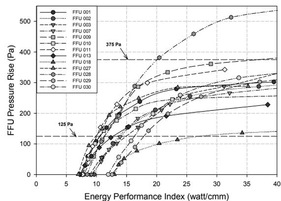
**Figure 4. 4'x2' FFU pressure rise vs. EPI (power intensity)**
