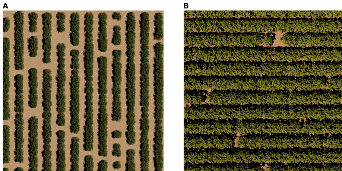
Fig. 7. Example large-scale simulated images. (A) Synthetic RGB image of part of the “Wellington Citrus Orchard” (extent 50 \times 50 \text{ m}^2 ) illuminated by a solar light source. The camera focal plane distance, HFOV, and diameter of the lens are 100,000 m, 0.143^\circ , and 0.01 m, respectively. (B) Synthetic RGB images of strawberry plants illuminated by a solar light source (extent 8 \times 8 \text{ m}^2 ). The camera focal plane distance, HFOV, and diameter of the lens are 11.5 m, 34.2^\circ , and 0.01 m, respectively.
