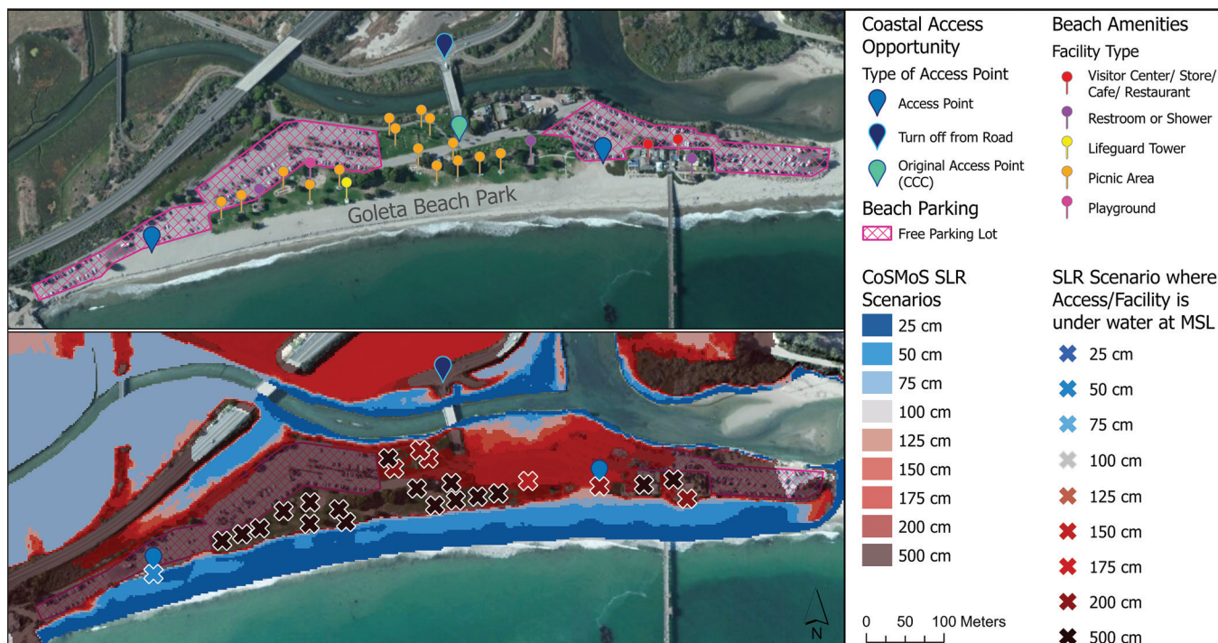
Figure 1. This two-panel figure illustrates a sample (Goleta Beach, Santa Barbara County) of how (top) access sites were virtually ground-truthed to identify exact locations of access opportunities, facilities, and amenities and how (bottom) SLR run-up models, generated by CoSMoS, were overlaid at 0.25 m intervals through 2.0 m and at 5.0 m to identify mapped locations that would be considered inundated. The original Coastal Access Database's single geolocation for Goleta Beach Park is indicated; all other features were created through virtual ground-truthing.
