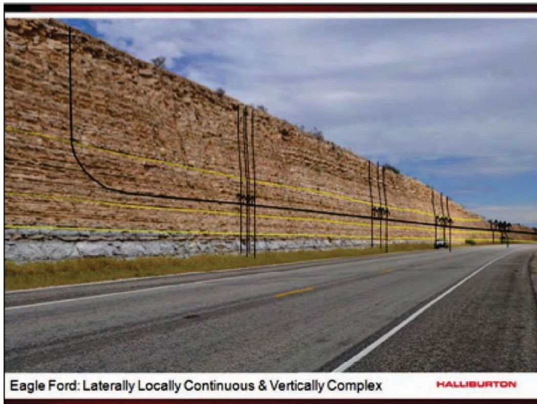
Figure 3.3-4. Schematic of a horizontal well with multi-stage hydraulic fractures superimposed on a road cut in the Eagle Ford Formation, west Texas (public domain image, courtesy of Halliburton 2013). The curved black line originating at the left represents a well bore turning horizontal. Potential locations for hydraulic fractures are indicated with vertical black lines. The yellow lines indicate depositional layers. The schematic demonstrates the lateral continuity of the Eagle Ford Formation, which lends itself to industrial-scale drilling of extended-reach horizontal production wells with multi-stage hydraulic fractures.
