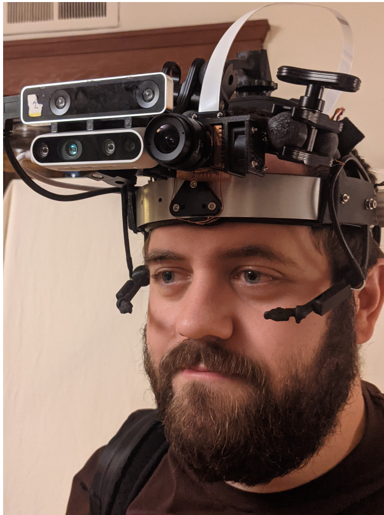
Figure 2.3: Subject wearing the device. The two scene cameras (Ximea and RGB-D) and tracker (IMU 1) are mounted together with a custom 3D-printed mount, adjustable in position with a 3-point ball-and-clamp adjustable mount. Custom ball-and-socket joints combined with set screws enable positioning of eye trackers below the eyes. A white ribbon cable connects the Ximea camera to the rear switch box.
