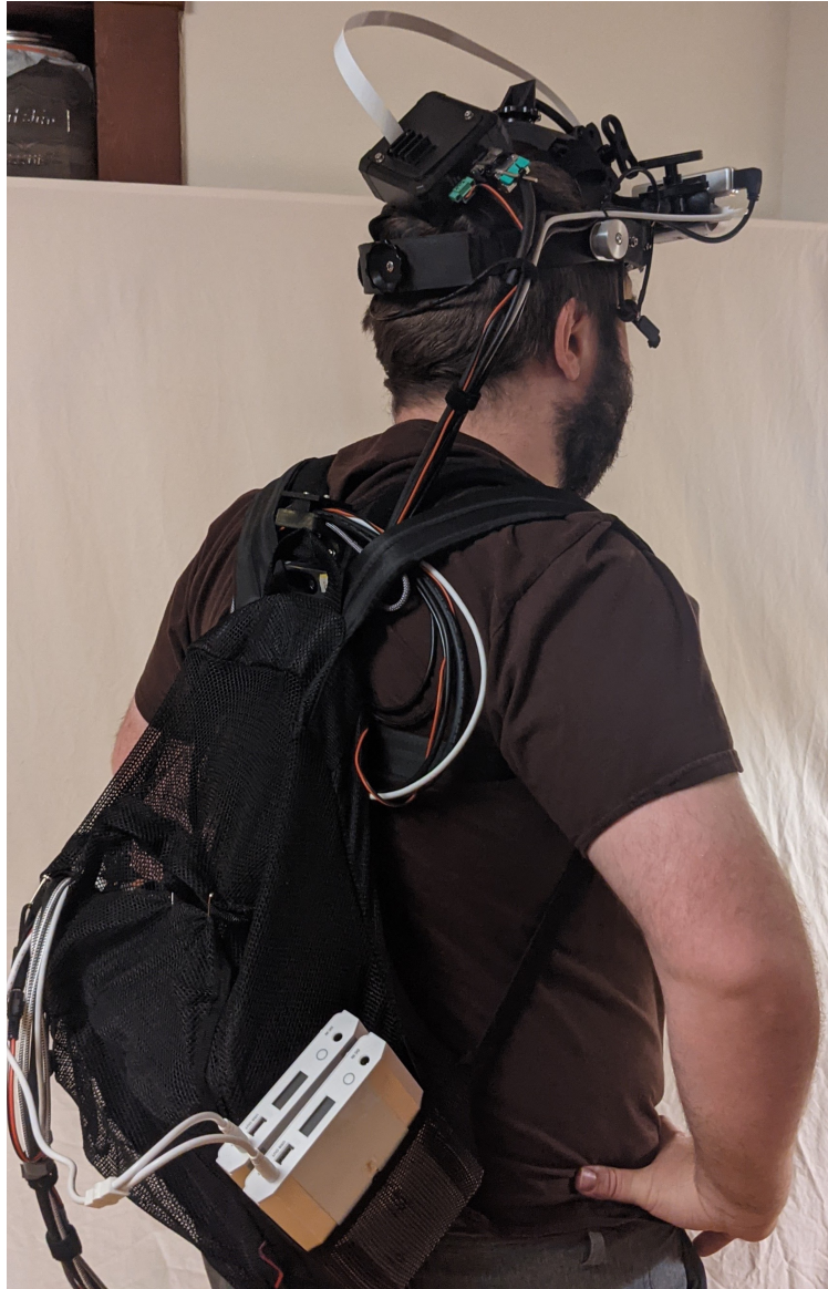
Figure 2.4: Rear view of a subject wearing the device with the backpack in mobile configuration. Computer and batteries are housed in the backpack. Ximea switch box is mounted with Velcro on the back of the head. Cords are bound in an adjustable loop enabling head mobility. Another motion tracker is mounted on back strap under backpack with the sensor positioned just above backpack.
