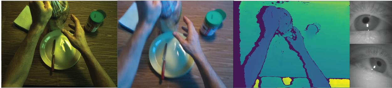
Figure 2.1: Left to right: Sample frames collected from Ximea camera, RealSense RGB stream, RealSense depth stream, and Pupil Labs binocular eye-tracking cameras. Images shown are frames as captured by each sensor, before post-processing.
