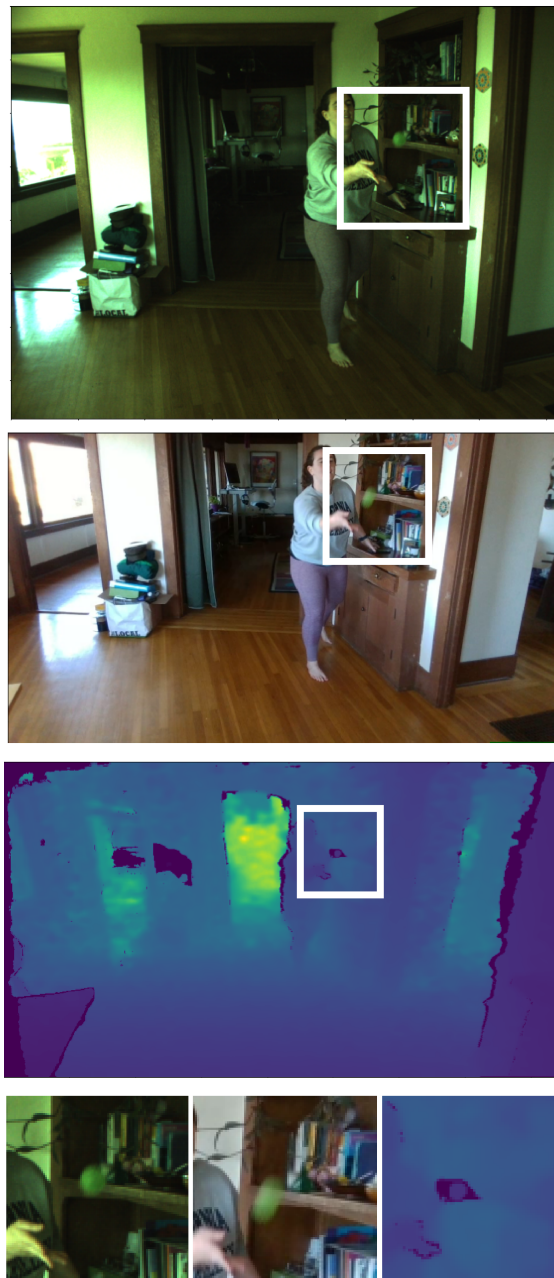
Figure 2.8: Visual streams are temporally synchronized to the framerate of the slowest visual stream (60Hz). Temporally synchronized frames from three visual streams (top to bottom): Ximea RGB stream, RealSense RGB stream, RealSense depth stream. White boxes indicate zoom-in on bottom panel, showing ball in same position at moment of release from hand during toss, which is evidence that timestamps are well matched. Note the greater motion blur of the ball in the RealSense RGB stream running at 60Hz (bottom middle panel) compared to the Ximea RGB stream running at 200Hz (bottom left panel).
