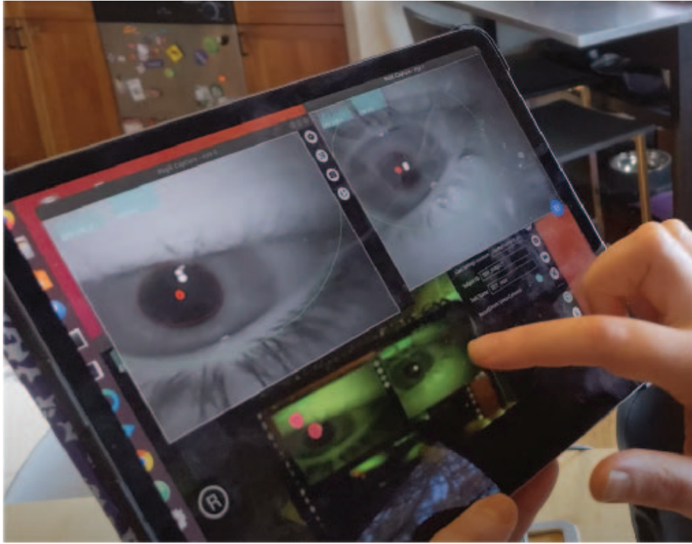
Figure 2.5: Hardware control during data collection is performed in Pupil Lab’s Pupil Capture with custom plugins running on the acquisition computer. The computer is controlled remotely with Chrome Remote Desktop over WiFi. Settings are adjusted and acquisition started and stopped by the experimenter using an iPad or laptop.
