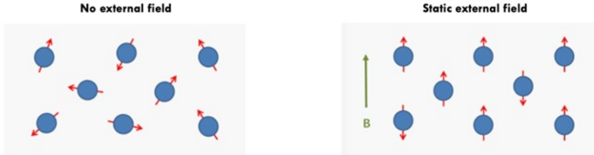
Figure 2.1: The influence of external magnetic field on the magnetic dipole in ferrimagnetic material.
