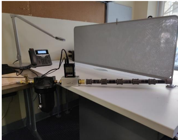
Figure 2.2 System used for repeatability tests- 1 ft of pipe with 10 unsealed joints
