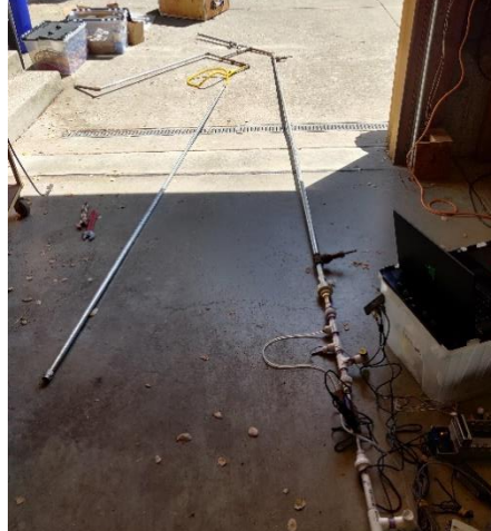
Figure 2.4 Leak testing apparatus connected to example pipe network used for testing aerosol sealing process
