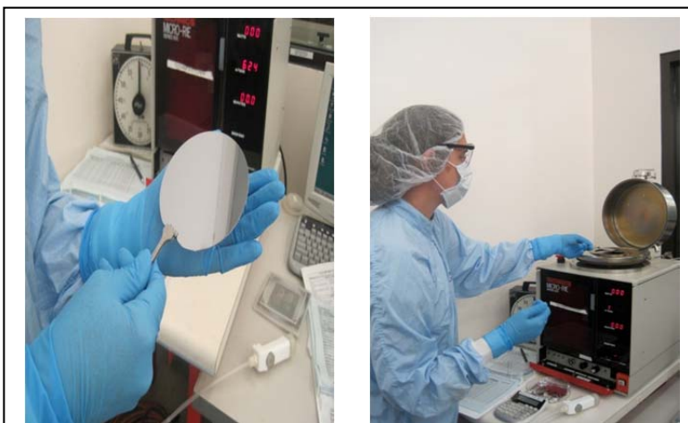
Figure 2: Clean room microengineering. Left: An example silicon wafer. Right: Substrates undergoing surface activation using clean room instrumentation.
