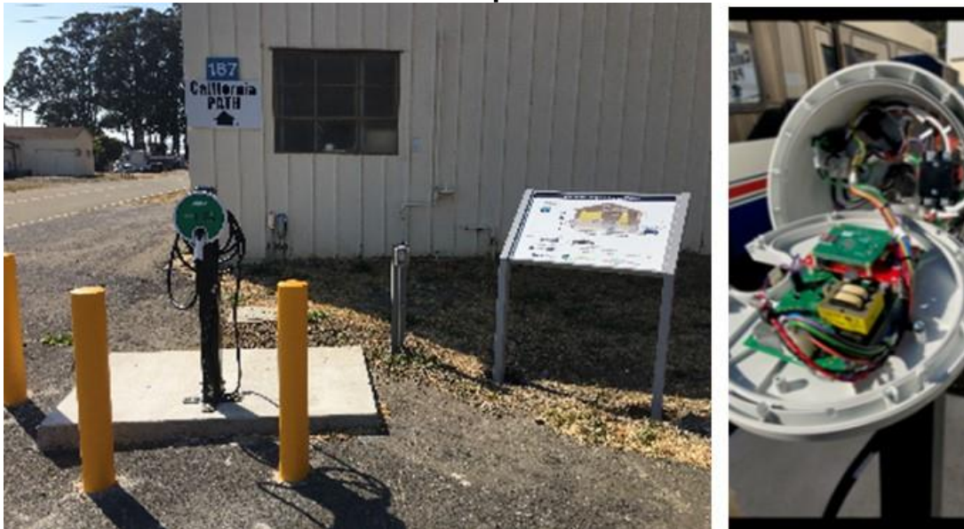
Figure D-1: VGI Test-Bed With Wi-Fi Enabled Charger at UC Berkeley Global Campus
