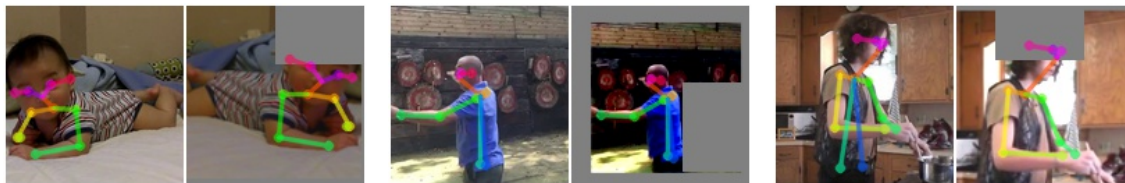
Figure 3.4: Data augmentation. We apply random spatial, cutout and color augmentations to frames and poses just prior to the discriminator network. Each pair above shows the original frame and pose on the left and the augmented output on the right.
