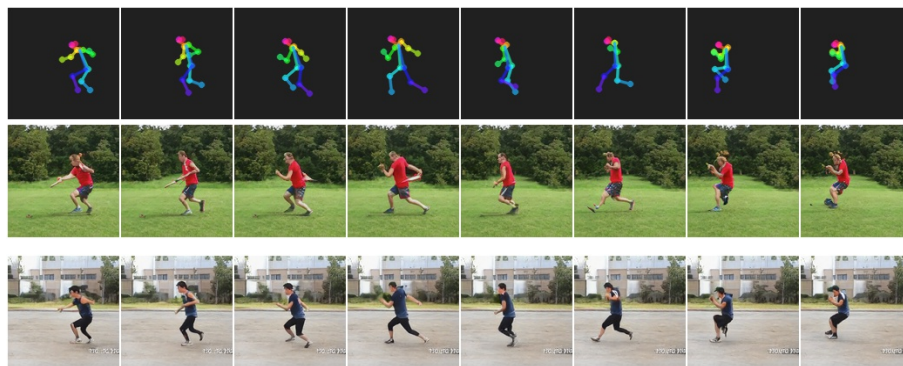
Figure 3.11: Provided an input pose sequence (top), we infer scenes based on the first pose, then generate animations (middle/bottom) by keeping the scene latent fixed and passing keypoint heatmaps for each subsequent pose.
