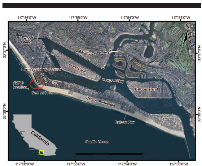
Figure 2. Berm experiments were conducted adjacent to Newport Pier in Newport Beach, California. Berms were constructed at low tide and exposed to runup and waves. The location of wave and pressure measurements (using AWAC) is shown. (Color for this figure is available in the online version of this paper.)
