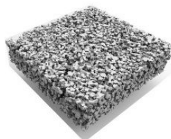
Porous Microstructure of S-NrGO Electrode
