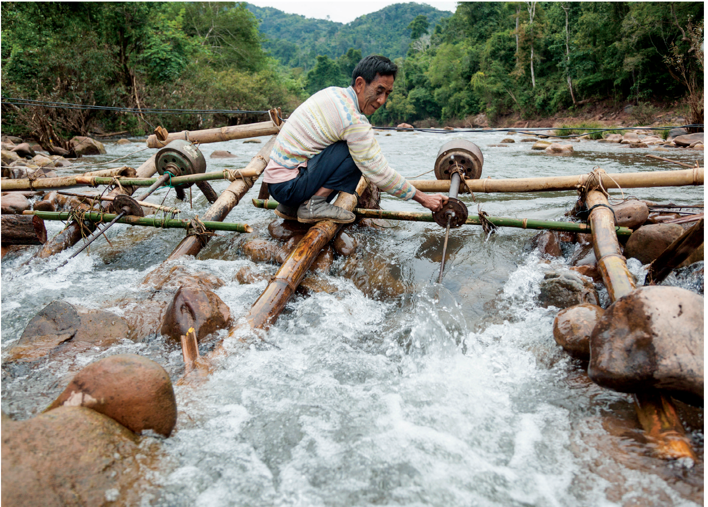
A microhydro turbine on the Nam Ou River in Laos generates electricity for nearby villages.
