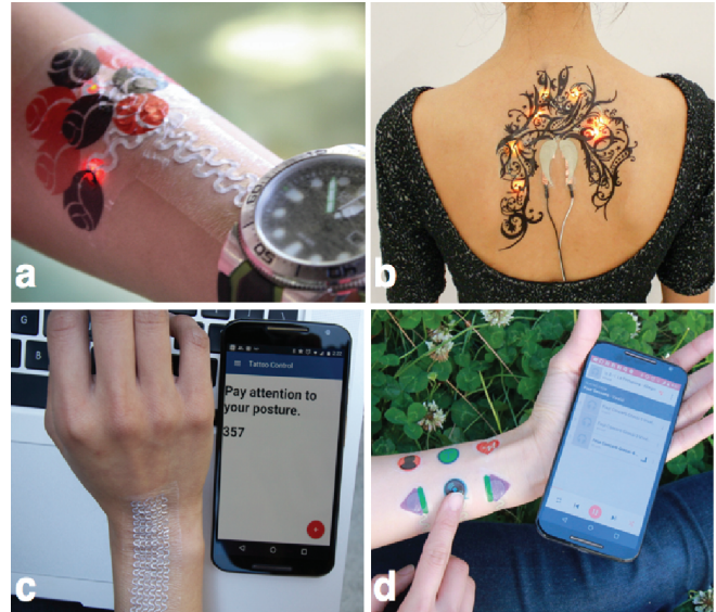
Figure 1. Skintillates is a class of temporary tattoo electronics that can be fabricated using an accessible process. a) A point-light display, b) A back tattoo LED display that flashes with music, c) A strain gauge that detects body position, d) capacitive buttons for mobile device control
