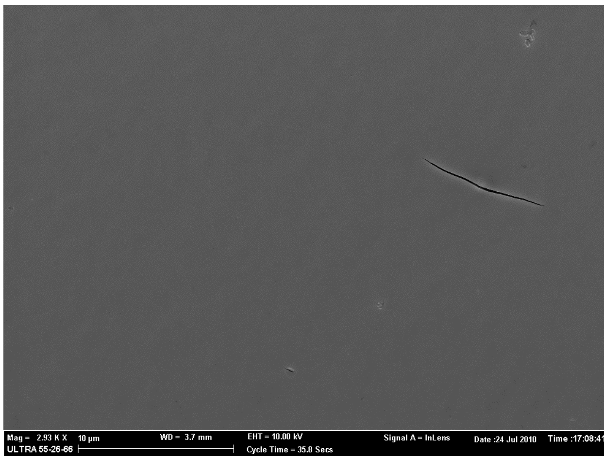
Figure 32 SEM Image of a CdSe nanocomposite film (6.1nm nanocrystal size). The image was taken near a crack to show that the image is in focus.
