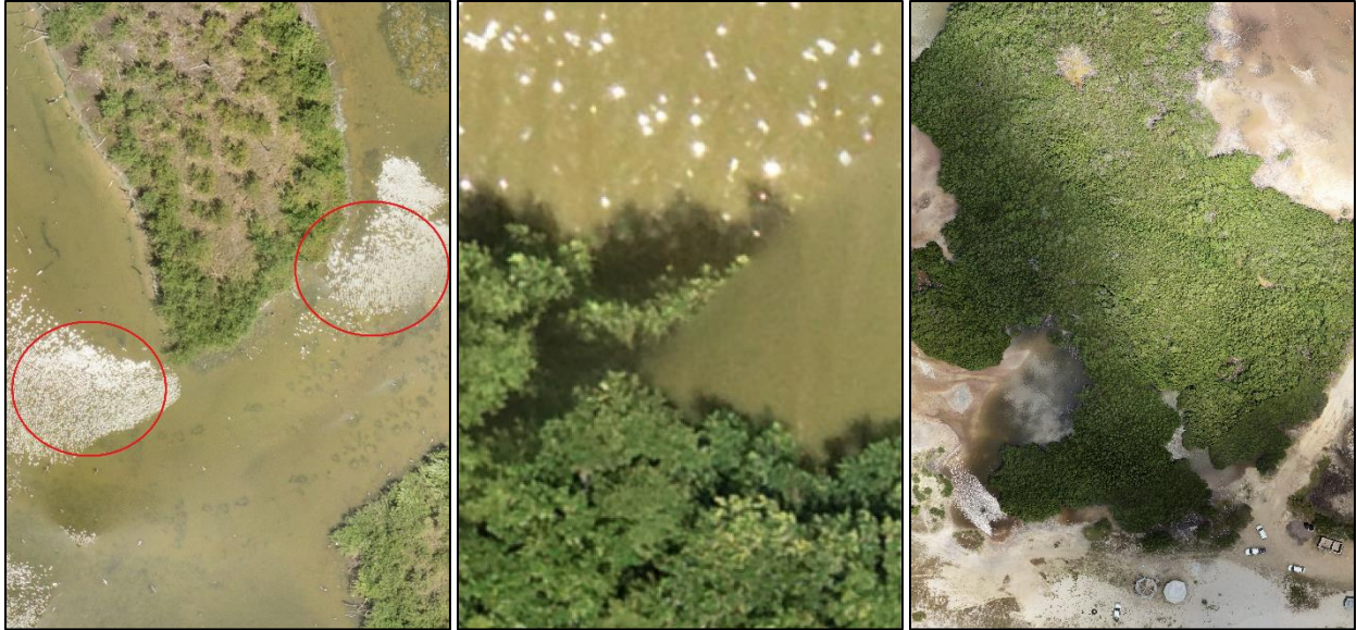
Figure 15 - Example selections of orthomosaics from the Jamaica Expedition. Pane 1: Sunspot reflections circled in red, Pane 2: orthorectification errors due to poor weather conditions, Pane 3: white balance inconsistencies due to intermittent weather conditions
