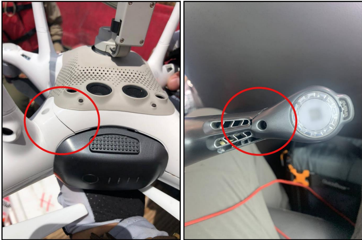
Figure 17 - Damage to two DJI Phantom 4 Pros during the Jamaica Survey due to high winds
