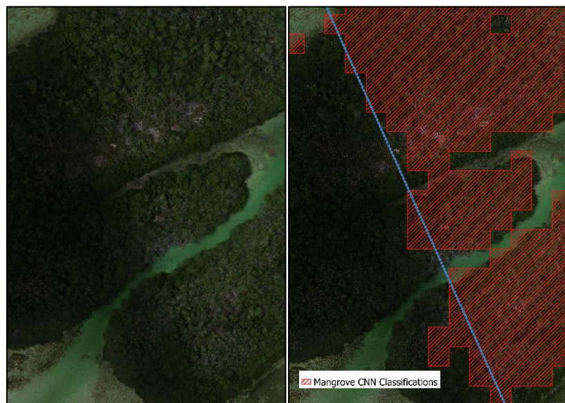
Figure 9 - Maps highlighting performance of CNNs with poor lighting; Pane 1 - Input mangrove drone image, Pane 2 - EfficientNet CNN Classifications
