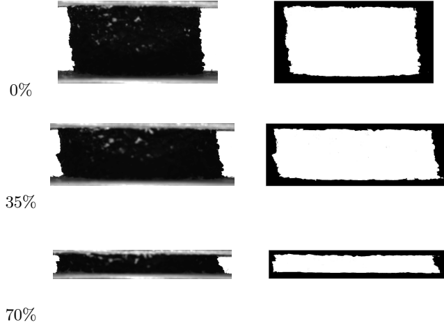
Figure 4: Original image from the digital camera vs Image after processing for TDM 600.
