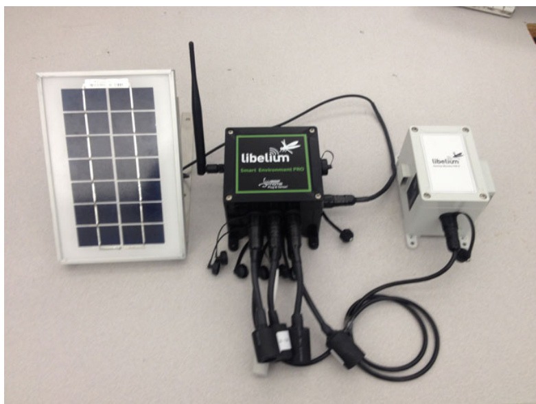
Figure 8.7: Libelium™ Smart Environmental Pro unit with wireless transceiver and solar power supply
