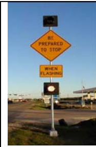
Fig. 7.1.1.1 Picture of a flashing beacon for end of green warning [7.6]
