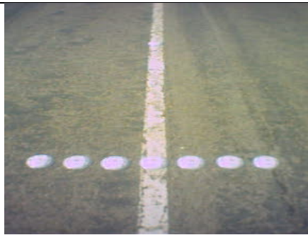
Fig. 6.2.1.1 The layout of 7 sensor nodes used for collecting magnetic signature array examples
