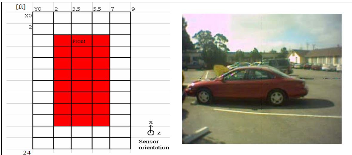
Fig. 5.2.2.1 Experimental layout (left) for the two dimensional magnetic measurement of a Ford Taurus 1996 (right)
