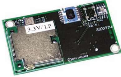
Fig. 7.2.1.1 Picture of MICA weather board MTS400 manufactured by Crossbow [7.24]
