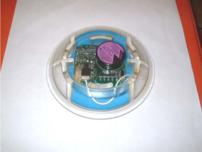
Fig. 3.2.1 Pictures of first generation prototype of the sensor node: TrafficDot
