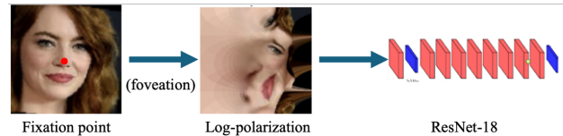
Figure 1: The Model 2.0 (TM2.0). The model includes sampling from the image via fixations (here, on the nose), driven by a salience map, followed by foveation, followed by log-polarization. This image is fed into a Convolutional Neural Network (CNN). To elucidate the role of the log-polarization, we compare this to the same model without it.
