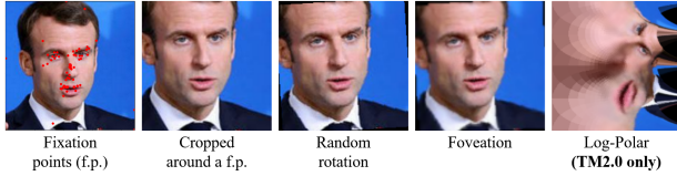
Figure 6: Data Transformation Pipeline. Fixation points are first gathered from each image. Then, centered on a sampled fixation point, each image is cropped, rotated in \pm 15^\circ , foveated, and log-polarized for TM2.0 only.
