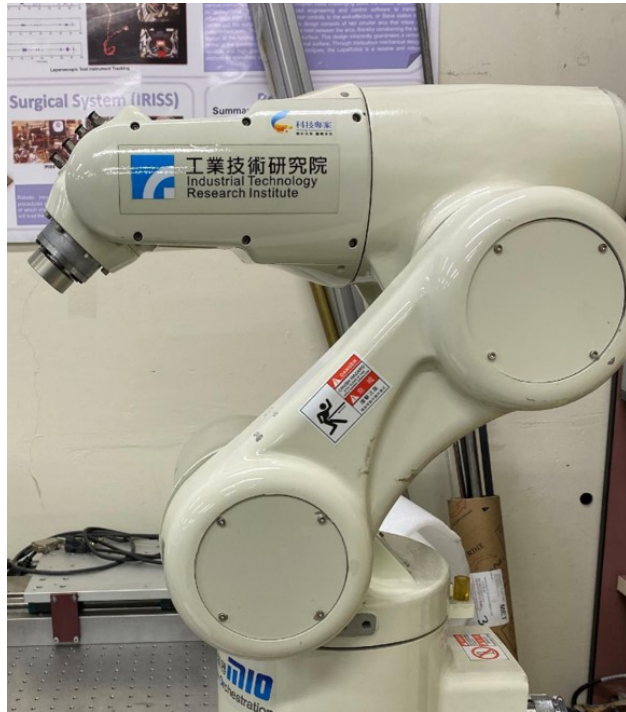
Figure 6.1: industrial robot AR-607 developed by ITRI
