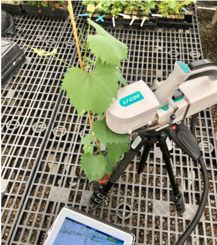
Figure 3. A portable photosynthetic system taking measurements prior to the beginning of the 28-day trial period
