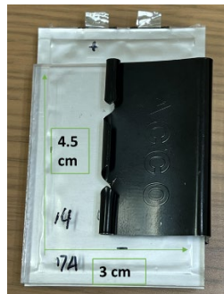
Figure 31. Optical images of a NMC622||LTO pouch cell.
