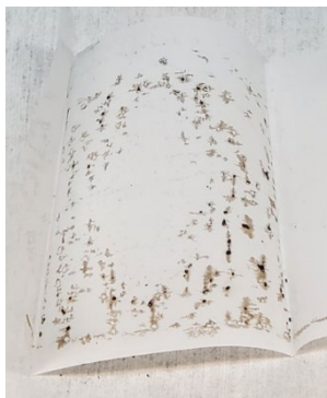
Figure 40. An optical image of lithium plating in NMC||Si pouch cell.
