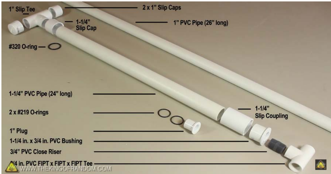
Figure A.12: Pump Design
