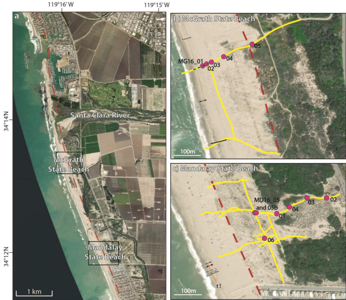
Figure 15. a) Overview of the study area, data collection sites labeled and outlined in black b) McGrath State Beach, and c) Mandalay State Beach. Red dashed line in all panels represents the 1855 shoreline. GPR profiles are shown by the yellow lines in panels b and c. Core locations are shown by pink dots and labeled. GPS profiles of the shoreline are shown by black lines. Transect t1 is shown by the orange line in panel c.
