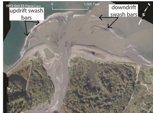
Figure 1. A) Schematic of mouth-bar deposition, and aerial image showing how the authors distinguished a mouth-bar. B) Swash-bar schematic and aerial image showing how authors distinguished swash-bars. (Schematic drawing by Scott Condon, and photos by A. Ritchie)
