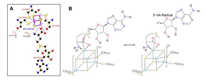
Fig. 1. (A)  $[Fe_4-S_4]$  binding motif from biotin synthase (PDB: 1R30). Image created using LigPlot+ (Laskowski & Swindells, 2011). (B) The common activation step associated with the canonical RSS.
