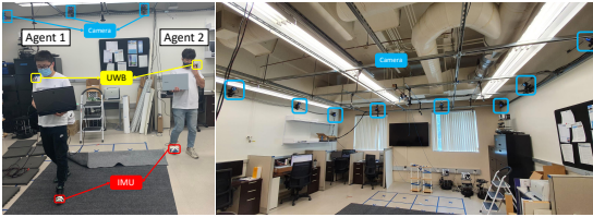
Figure 7 – The test experiments for LDMV and LPECMV conducted in the KCS lab with the aid of the OptiTrack motion capture system.
