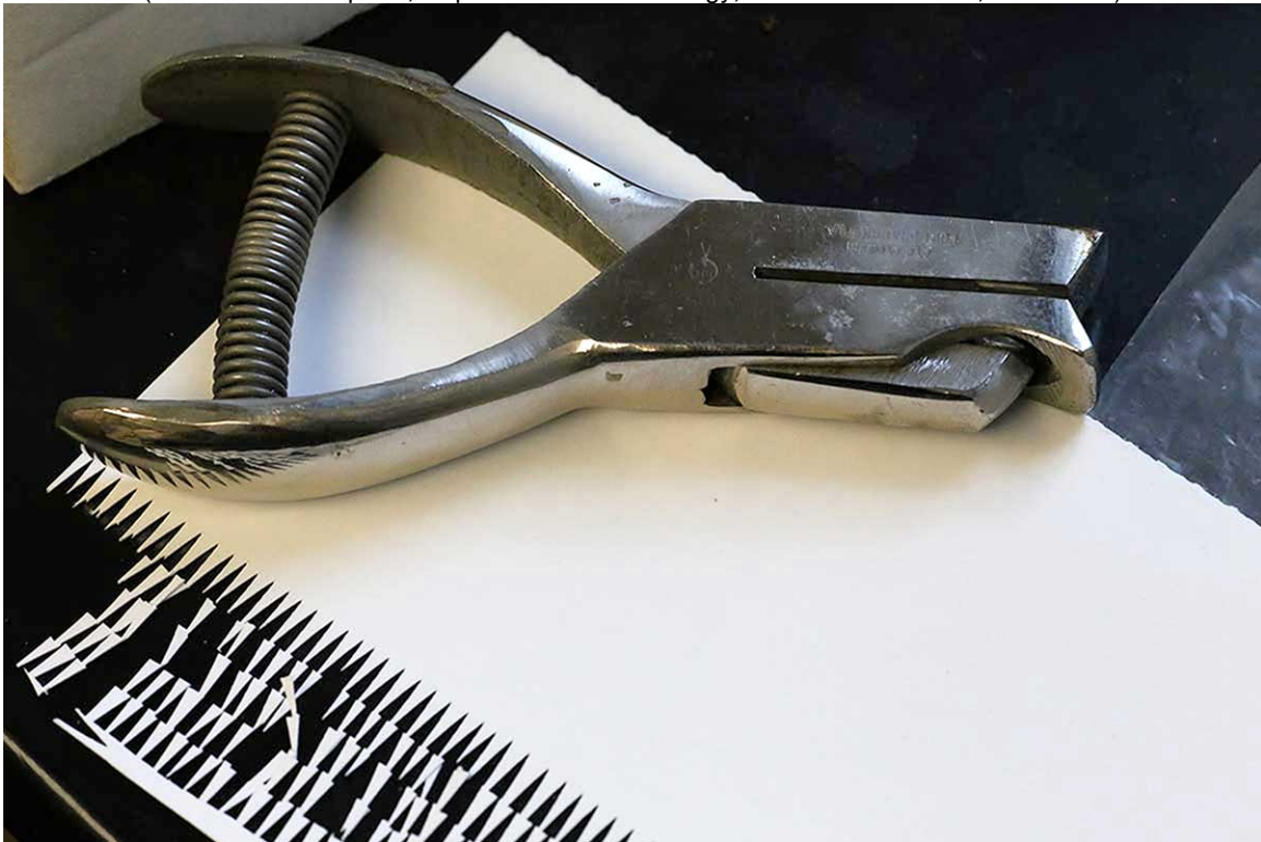
Figure 6-41. Point punch and acid-free cardstock (Division of Coleoptera, Department of Entomology, Smithsonian NMNH, June 2015)
