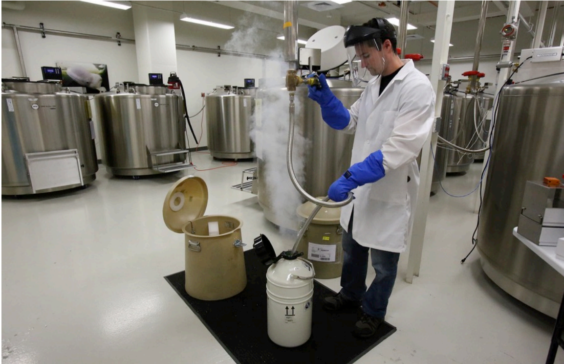
Figure 4-13. GGI “tube wrangler” Steve Thornton filling a liquid nitrogen dewer. (Smithsonian Biorepository, December 2014)
