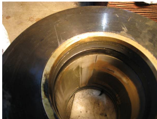
Figure 79. View of Inside of Bearing Showing Scratches From Abrasion as well as a Vertical Seam
