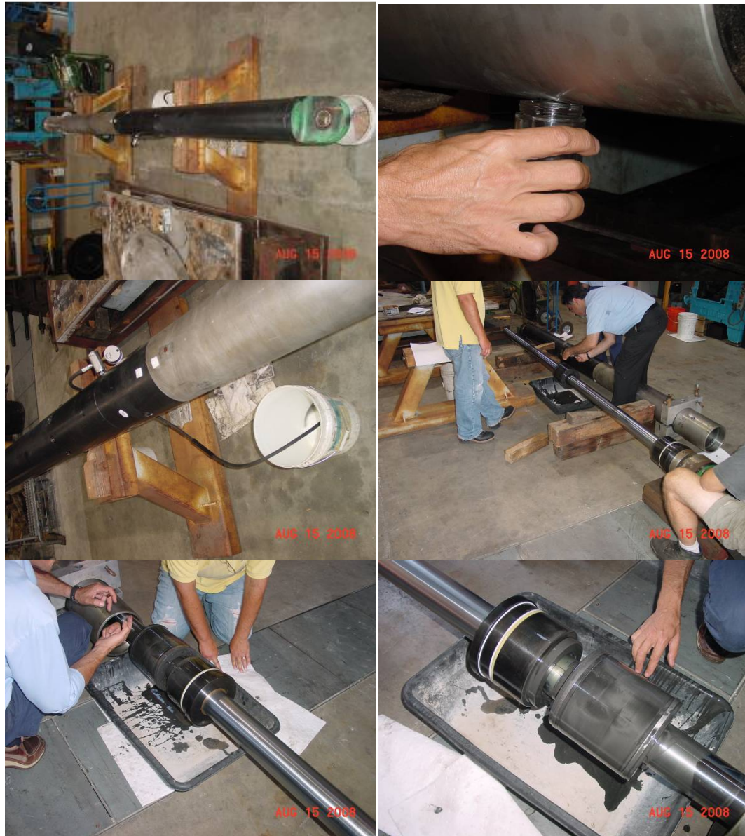
Figure 75. Disassembly of the Damper
