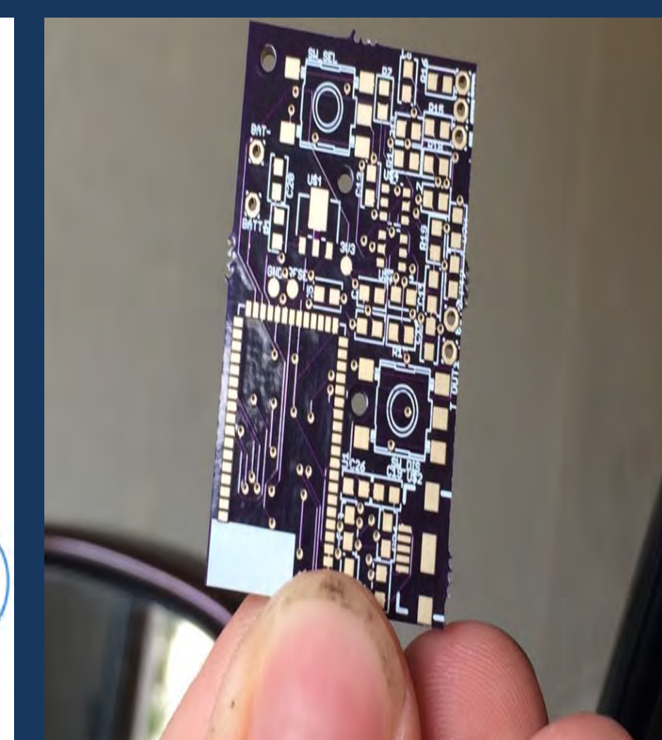
(left) Block diagram of our overall system (right) Our unpopulated PCB
