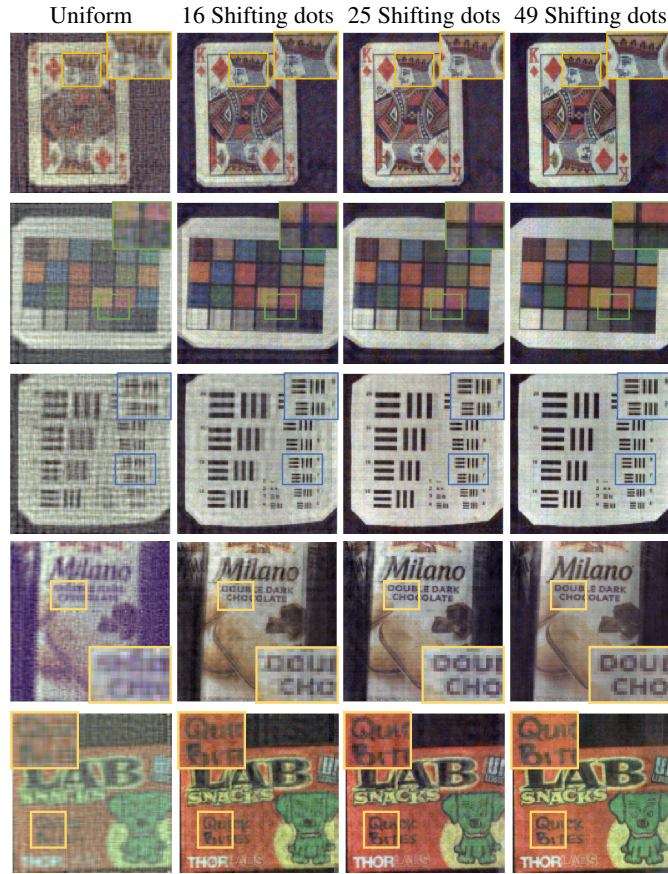
Figure 4.7: Experimental results on five test scenes with different numbers of shifting dots patterns. The reconstruction results using multiple coded illumination patterns outperform the standard lens-less camera with uniform illumination. The quality of reconstruction gradually increases as the number of illumination patterns increases.
