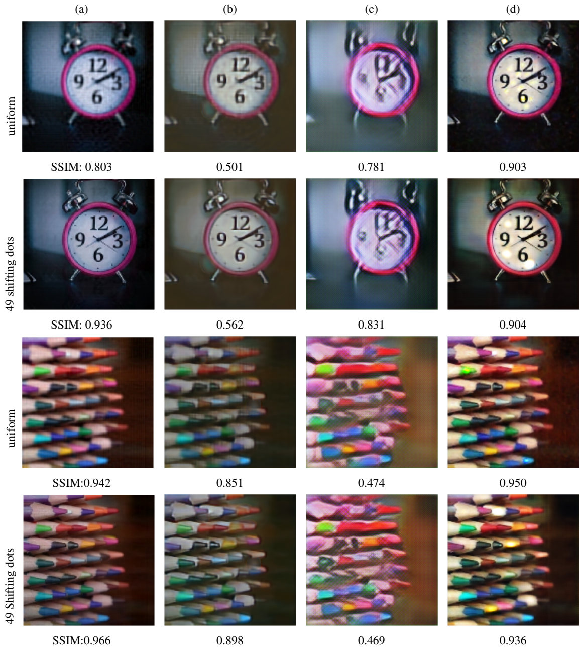
Figure 4.12: Reconstruction results for simulated measurements with 49 uniform and shifting dots illumination patterns. Images in four columns show (a) LS solution, (b) LS solution with trained UNet refinement, (c) LS solution with pretrained FlatNet refinement, and (d) trained FlatNet that reconstructs image directly from measurements. For each image, we show the SSIM value underneath.
