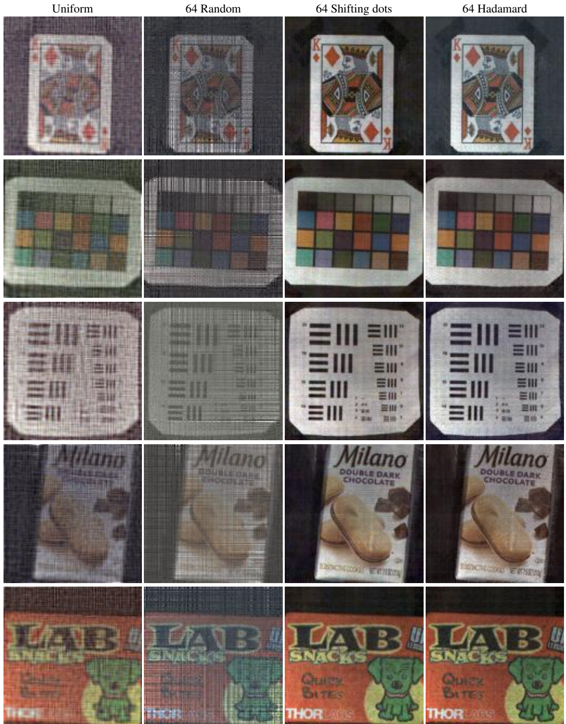
Figure 4.8: Experimental results on five test scenes with different types of illumination patterns. The orthogonal patterns (shifting dots, hadamard) outperform random patterns and uniform illumination.
