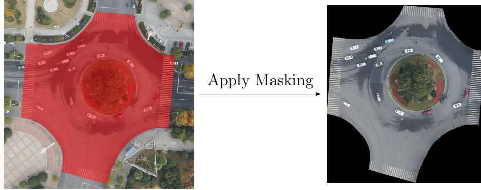
Figure 4.8: A demonstration of the masking process. The red polygonal mask is defined via CVAT. Pixels outside of the mask are considered irrelevant and are marked as black.
