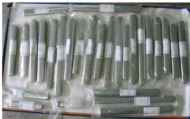
Fig. 2 Final inventory after the zone-refinement of the enriched germanium used for the production of the GERDA Phase II detectors
