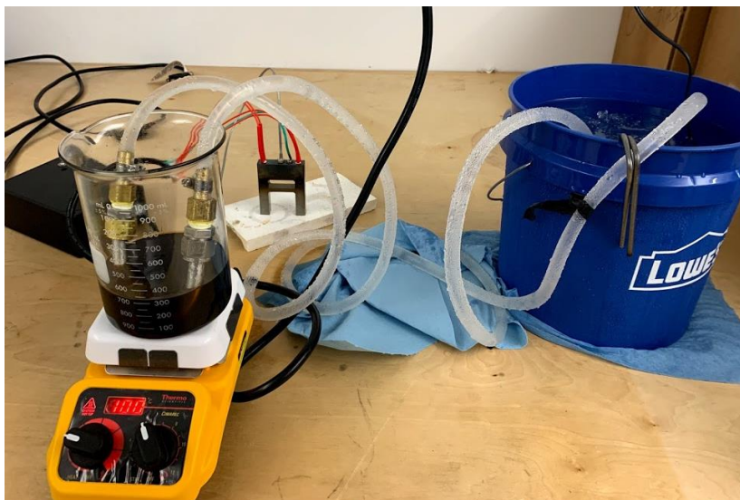
Figure 4-5: Thermal test set up, hot plate set at 100° C with magnetic stir simulating flow and 0° water circulating through the steel U-bend.
