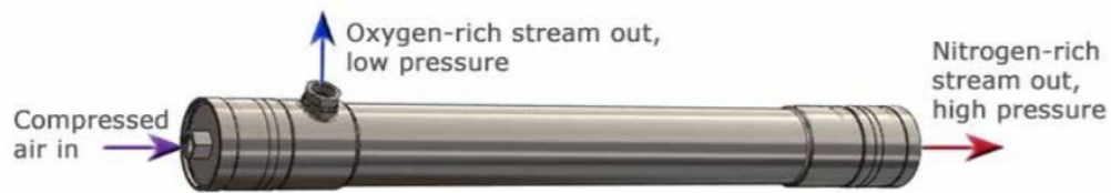
Figure 3: Oxygen filter from PRISM that removes 40% of oxygen and allows for a nitrogen rich air stream
