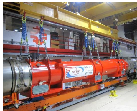
Fig. 1. Installation of LQXFA/B02 at Fermilab’s horizontal test stand.
