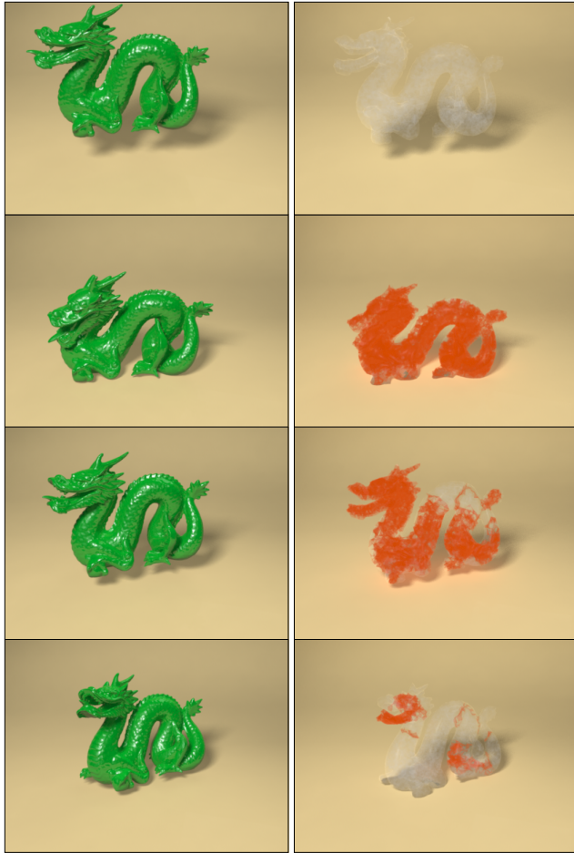
Fig. 4: The images in the left column are taken from an animation of a deformable dragon model dropped onto a flat surface. The dragon compresses and then bounces. The images in the right column indicate in orange the locations of the elements that are being updated.
