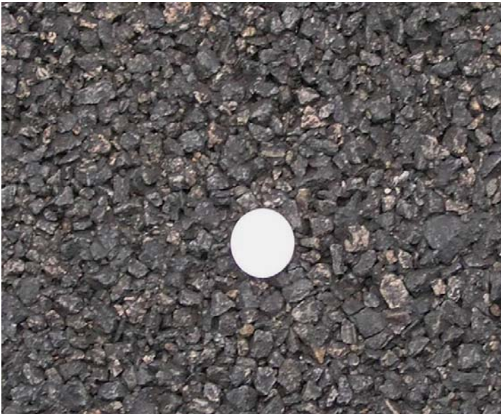
Figure 12: Open-graded asphalt concrete (OGAC).
