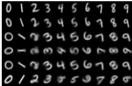
Figure B.2: VAE samples conditioned on different values of y (x axis) and z (y axis). The VAE learns to use z to represent rotations.
