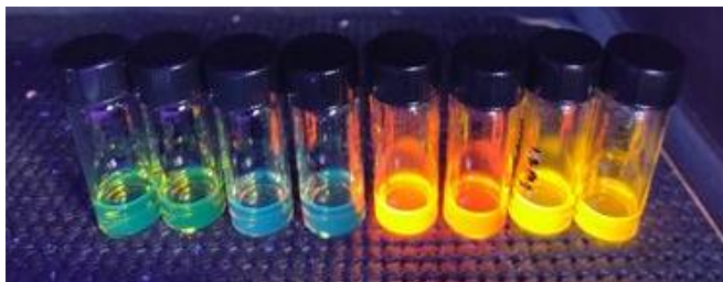
Figure 3.A.2. Image of EAT08 analogues in solution. Analogues are dissolved to a concentration of 4 mM in DMSO. From left to right: EAT08, EAT08-P, EAT08-A, EAT08-AP, EAT08-N, EAT08-NP, EAT08-NA, EAT08-NAP.
