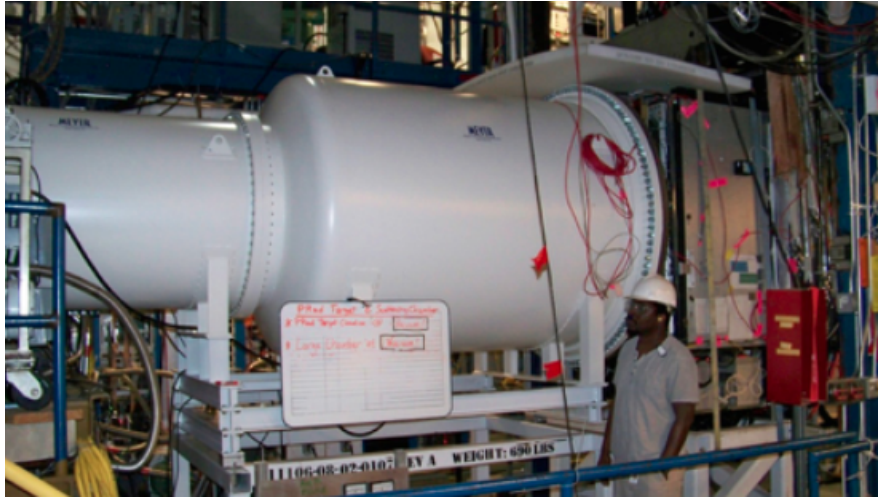
FIG. 15: A photograph of the \sim 5 m long, two stage vacuum chamber used during the PRad experiment (left). A photograph of the 1.7 m diameter thin window at one end of the vacuum chamber (right). Here the GEM and HyCal have been moved downstream for technical service.
