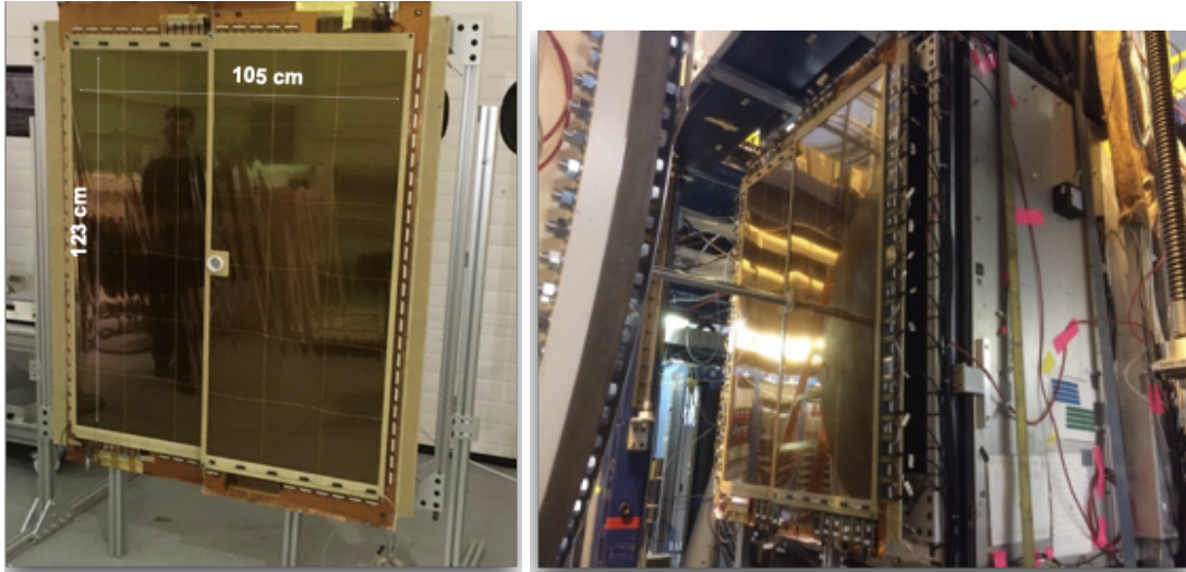
FIG. 19: The PRad GEM chambers (left) and the GEM chambers mounted on the HyCal during the experiment (right).
