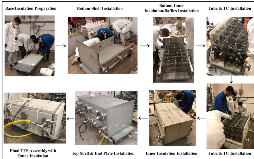
Figure 2D - Pilot demonstration system assembly
