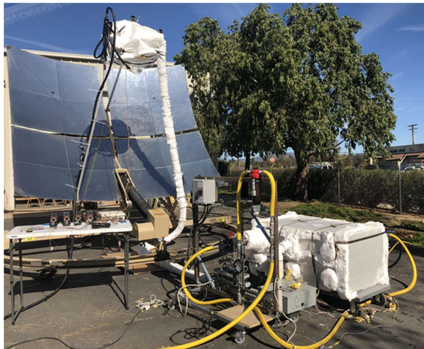
Figure 19 - Pilot scale SulfurTES demonstration system with CSP-dish collector [33]
