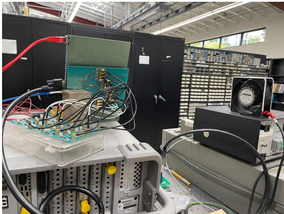
Fig. 7.22: RF Board Connected to LO Board with MCX Cables
