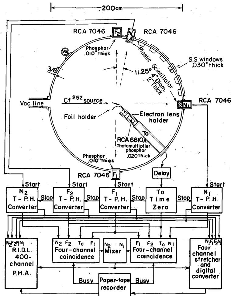
Fig. 1. Block diagram of the apparatus used to measure the velocities and angular distribution of prompt neutrons relative to the direction of the fission fragments.
